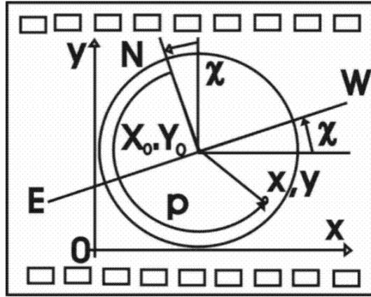
**Figure 2:** Angle  $\chi$  between daily parallel and horizon, which needs to be calculated.
