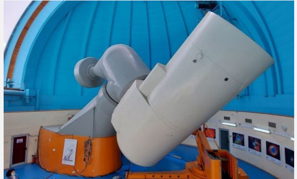
2m telescope with mounted ESPERO Echelle spectrograph
