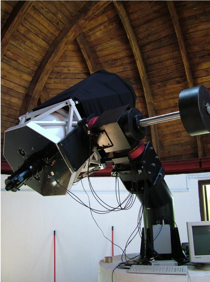
**Figure 4:** The 60 cm telescope at ASV.
