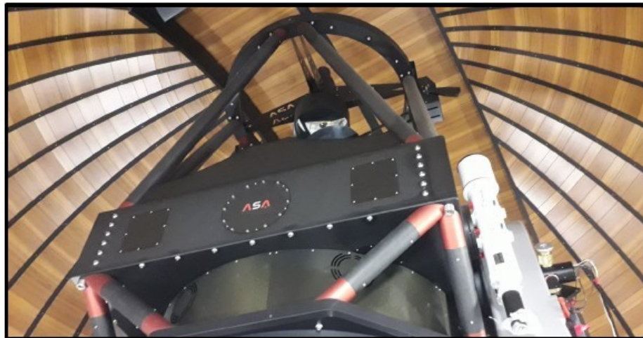
Figure 1. The ASV 1.4 m telescope in dome.
