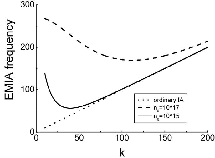
Figure 1: The electromagnetic ion sound frequency in units of  $\kappa_n c_s$  for the two number densities  $n_0 = 10^{17} \text{ m}^{-3}$  (dashed line), and  $n_0 = 10^{15} \text{ m}^{-3}$  (full line) in terms of  $k$  normalized to  $\kappa_n$ .
