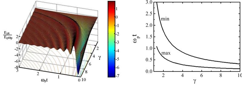
Figure 2: (a) Reflected EM field in time as a function of the plasma velocity  $\gamma$ . (b) Time period of the first and second peak in the reflected wave versus plasma velocity.
