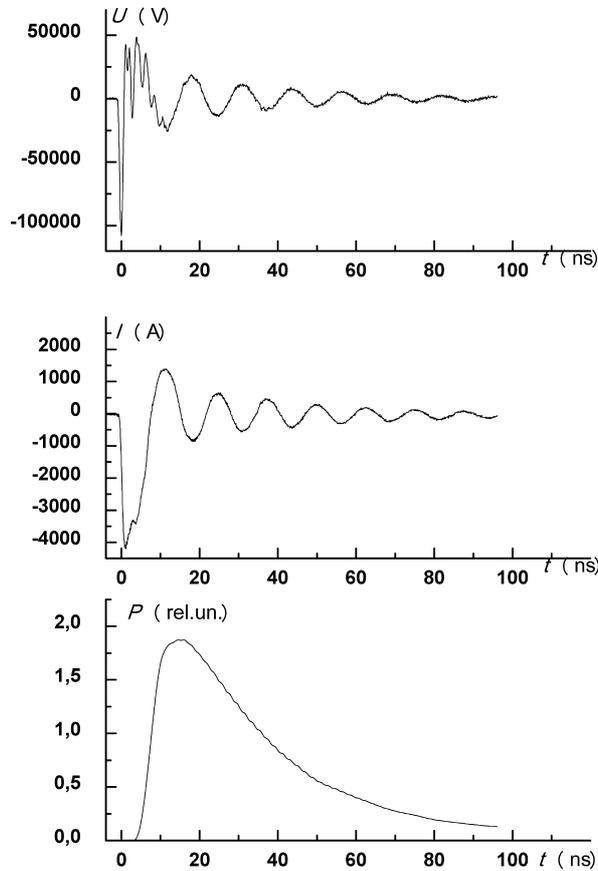
Figure 4: Typical oscilloscope traces of voltage pulse, discharge current and light pulse of volume discharge in Xe/Br<sub>2</sub>=50/1 working mixture at 500 Torr.
