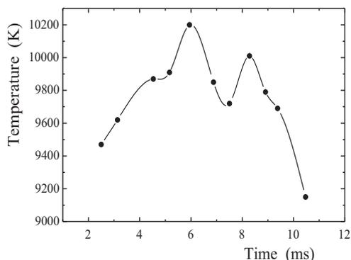
Figure 6: Temporal dependence of the plasma jet temperature.
