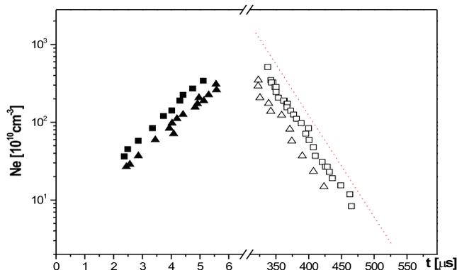
Figure 2: Measurement of the electron density at two position close to each other, from the top port:  $x=48\text{mm}$ ,  $y=4\text{ mm}$  (square) and from the side port:  $x=50\text{mm}$ ,  $y=0\text{mm}$  ( $\Delta$ ). Full and empty symbols represents creation and decay phase, respectively. The dotted line represent extrapolated curve for position  $x=48\text{ mm}$  and  $y=0\text{ mm}$ .
