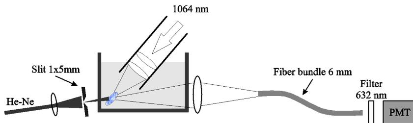
Figure 1: Experimental lay-out for forward scattering measurements.
