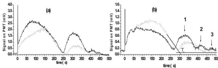
Figure 2: Signal from the light scattered at  $90^\circ$  on the gas bubble produced by the laser with pulse energy  $65 \text{ mJ}$  (dots) and  $280 \text{ mJ}$  (solid): a) without slit; b) with slit;  $T_c$  is measured first collapse period at lower energy; 1-3 indicate the bubble rebounds at the higher laser energy.
