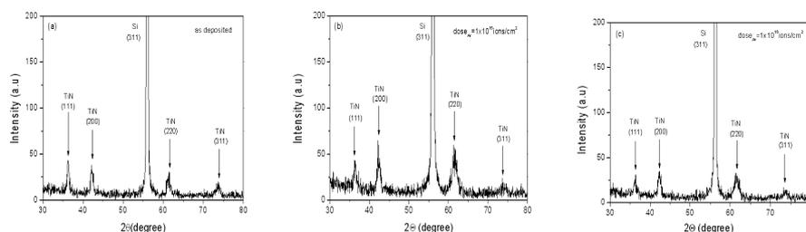
Figure 3: XRD analysis of TiN/Si samples: a) as-deposited, b) after ion irradiation to  $1 \times 10^{15}$  Ar/cm<sup>2</sup>, c) after ion irradiation to  $1 \times 10^{16}$  Ar/cm<sup>2</sup>.
