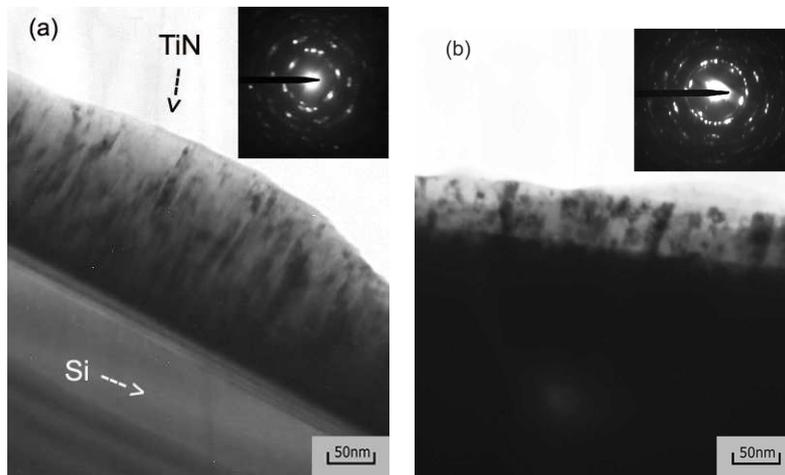
Figure 2: TEM analysis of samples: a) bright field image of as-deposited, b) bright field image of implanted to  $1 \times 10^{16}$  Ar/cm<sup>2</sup>.
