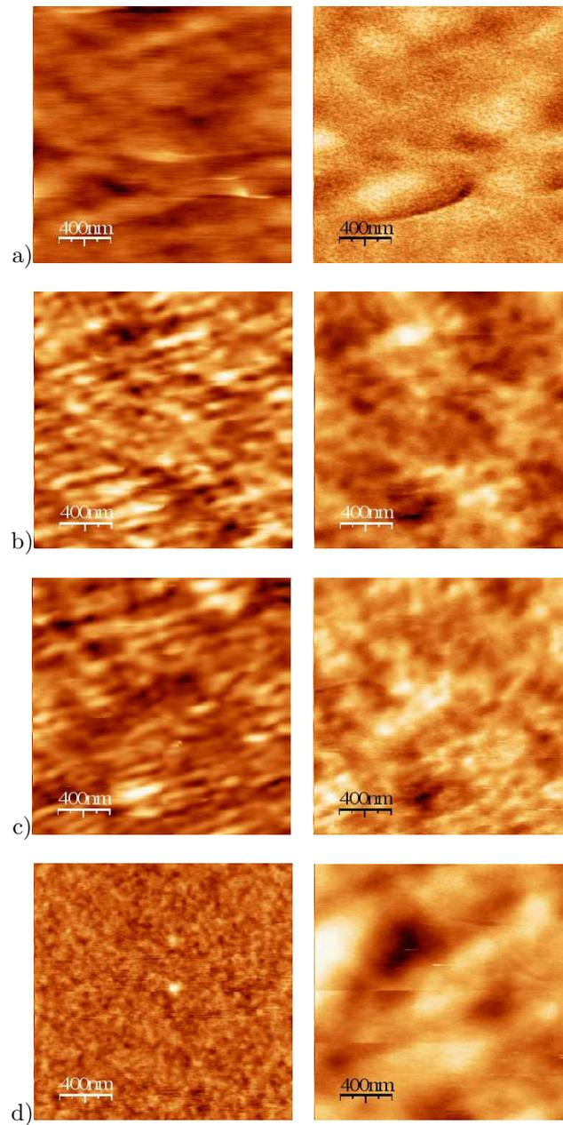
Figure 1: (a-d) Topography(AFM) images (left) and MFM images (right) of Co/Si bilayers: (a) as deposited; (b) irradiated to  $5 \times 10^{15}$  ion/cm<sup>2</sup>; (c)  $10 \times 10^{15}$  ion/cm<sup>2</sup> and (d)  $15 \times 10^{15}$  ion/cm<sup>2</sup>.
