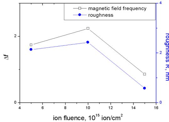
Figure 2: The Xe ion fluence dependence of magnetic frequency ( $\Delta f$ ) and roughness (R) of Co/Si bilayers irradiated with  $5 \times 10^{15} \text{ ion}/\text{cm}^2$ ,  $10 \times 10^{15} \text{ ion}/\text{cm}^2$  and  $15 \times 10^{15} \text{ ion}/\text{cm}^2$ .
