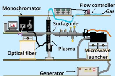
Figure 1. Experimental Setup
