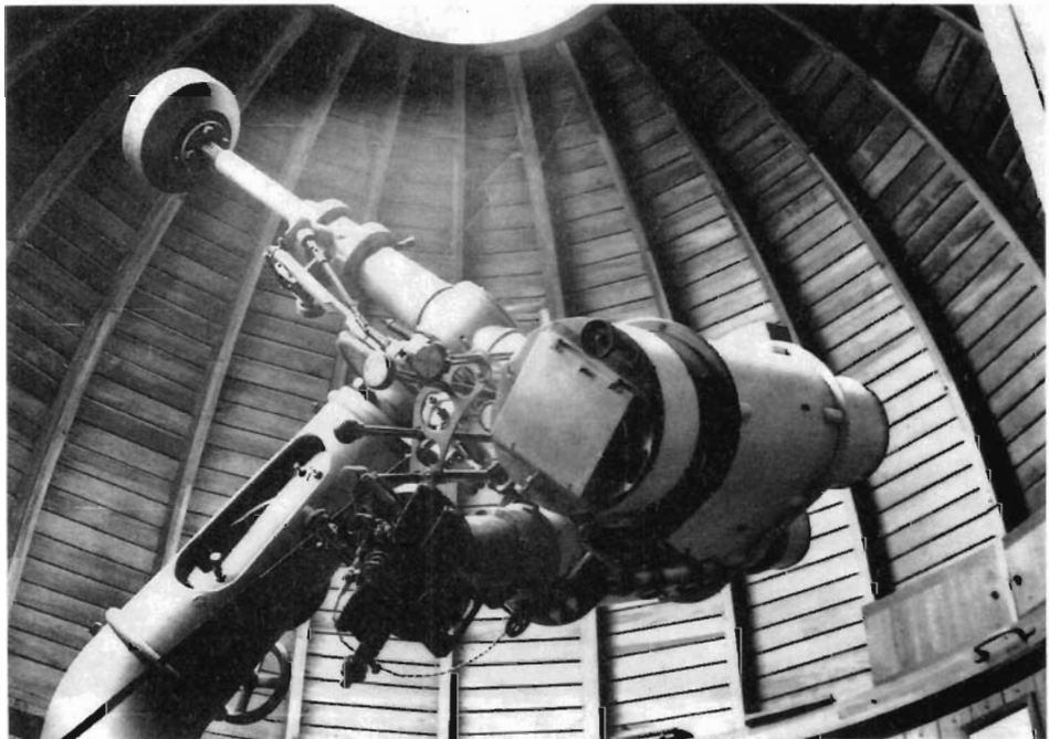
Fig. 10. Photovisual refractor "Ascania" 135/1000 and 125/1000 mm.
